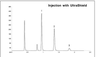
As the above chromatograms illustrate, UltraShield Precolumn Filters maintain the theoretical plates, N, of very efficient UHPLC columns. Column: 4.6 x 50 mm HALO<sup>®</sup> C18 Fused-Core<sup>®</sup>
