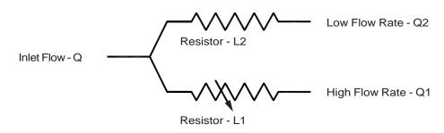
L1 = Adjustable fluid resistor (metering valve)
