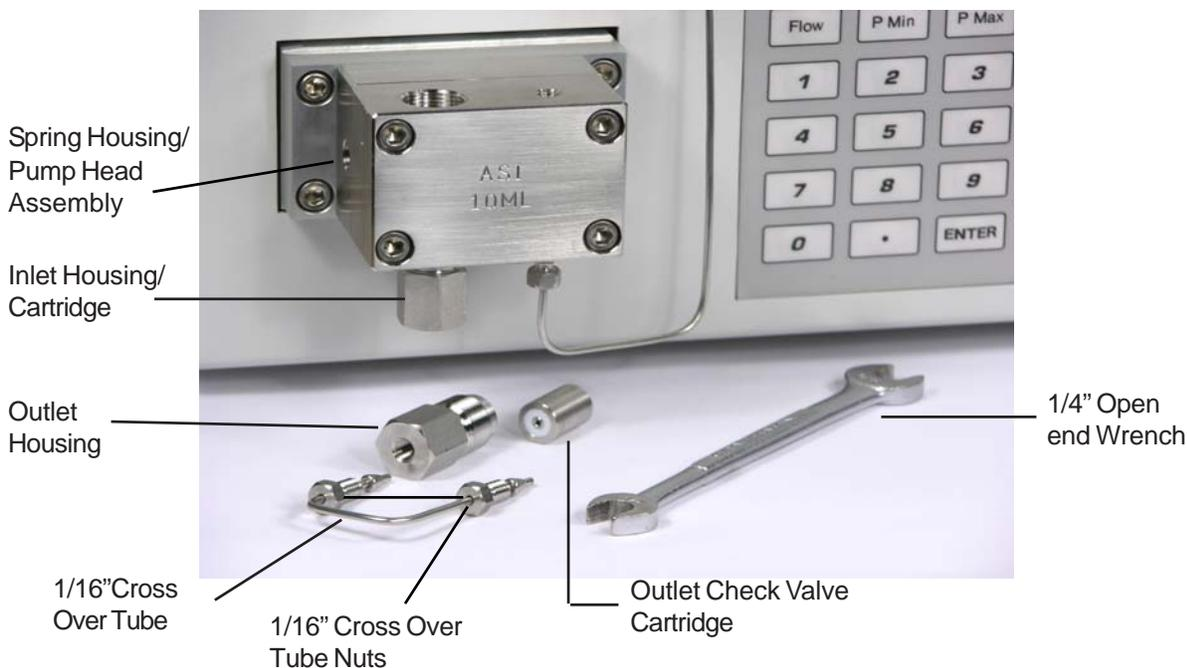
Figure 8. Check Valve Replacement.
