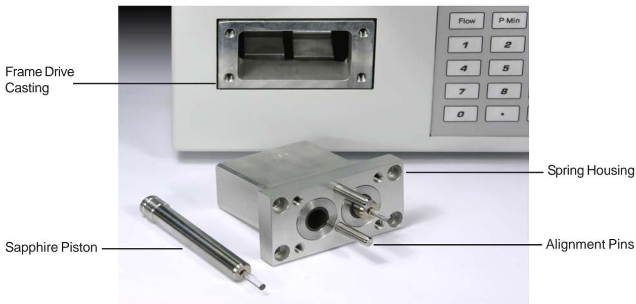
Figure 11. Sapphire Piston Replacement
